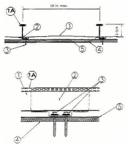
1. **Metal Roof Deck Panels\*** — No. 24 MSG min. thick coated steel, 16 in. wide max, 2-3/4 in. high at the side ribs. Steel batten (Item 1A) used over panel side ribs. Panels continuous over three or more clips. Side ribs to be seamed continuously with a special seaming tool with seaming operation to include panel clips (Item 2) and panel batten. End laps to be 6 in. wide. Panels may be mechanically curved to a minimum of 30 ft radius.
