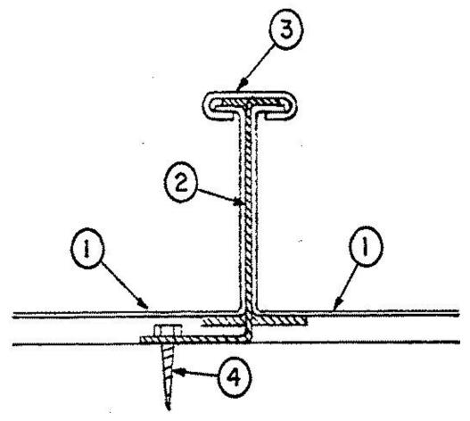
1. **Metal Roof Deck Panels\*** — No 24 MSG coated or stainless steel max, width 16 in., 2-3/4 high at side ribs. Panels continuous over two or more spans. End laps to occur near purlin supports with panels overlapped 6 in. Panels may be mechanically curved to a minimum of 20 ft radius. A bead of sealant may be used at panel side ribs and end laps. Side ribs to be continuously seamed with a special seaming tool with the seaming operation to include panel clips and panel batten.
